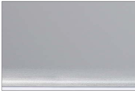
ClearMatt®- 0.250 mils (6 micron) film thickness - 180° bend - 2t (2 mm) radius -
