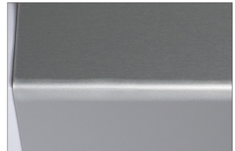
ClearMatt® - 0.425 mils {19 micron} film thickness - 90° bend, 2t {2 mm} radius
