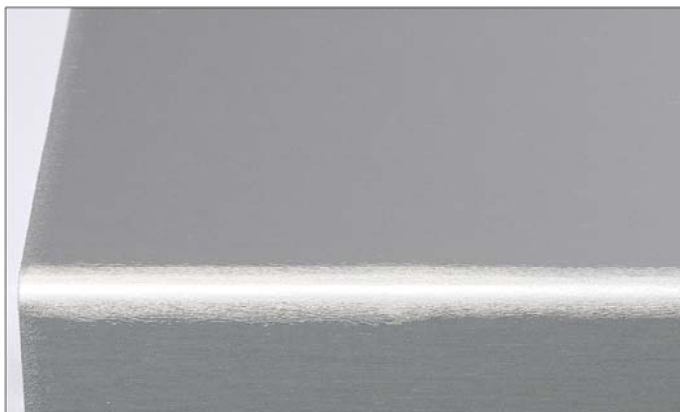
ClearMatt® with a 0.750 mils {19 micron} film thickness - 180° bend - 0t radius -
