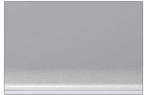
ClearMatt®- 0.750 mils (19 micron) film thickness - 180° bend - 2t (2 mm) radius -
